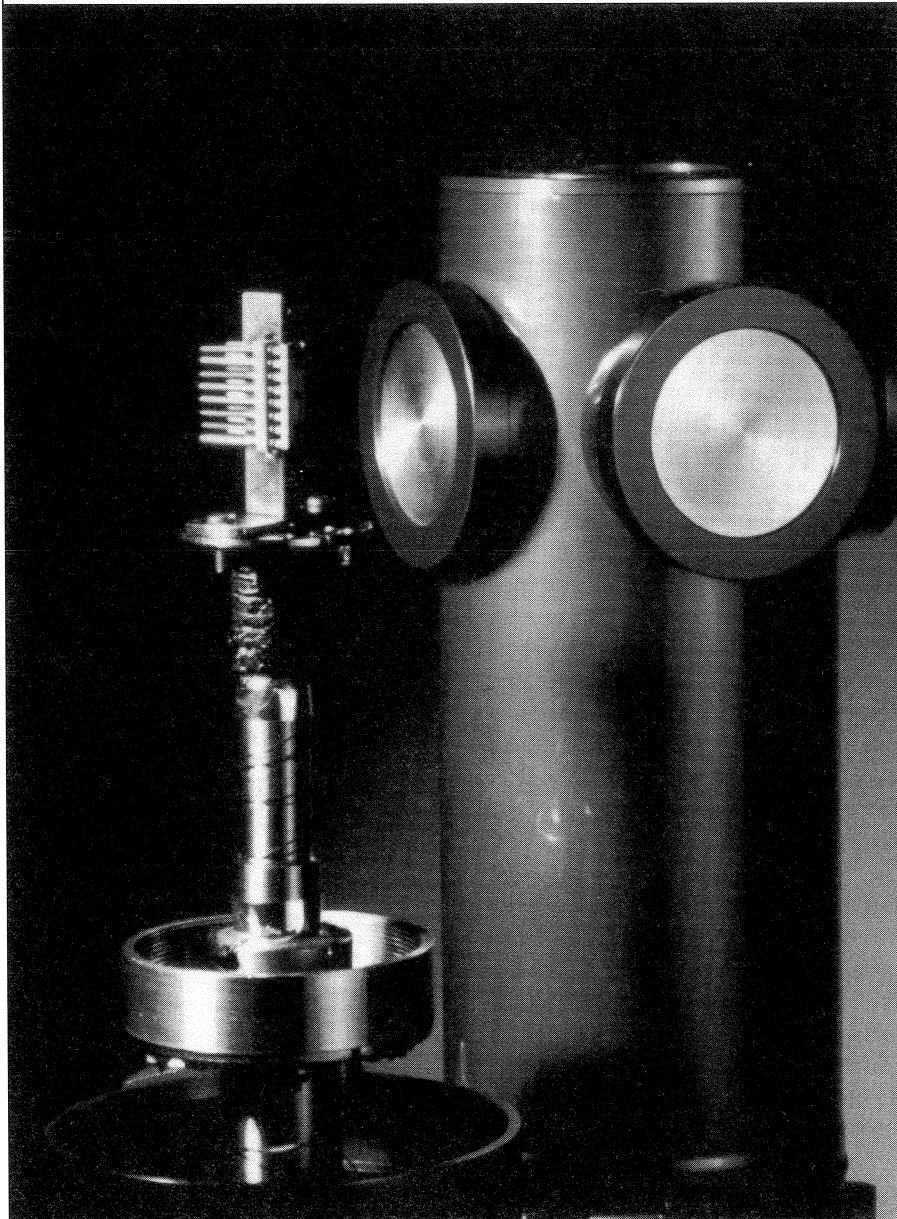
A circuit consisting of transistors of dimensions smaller than 1 micron is shown mounted in a cryostat for measurements of the electrical characteristics and noise as a function of temperature. An important result of the NOISE Action (3017) is that the ageing of transistors is accelerated at low temperatures, thus providing new means for addressing problems of balance between performance enhancement and degradation. (Photo: B. Ciancia, LPCS, Grenoble)
