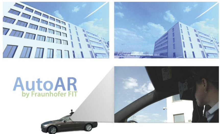
Figure 1: Auto AR system allows the user to experience virtual building models on site. Photo: Fraunhofer FIT, VWFS, Oltmanns und Partner, DhochN, Büro Gaudlitz.
