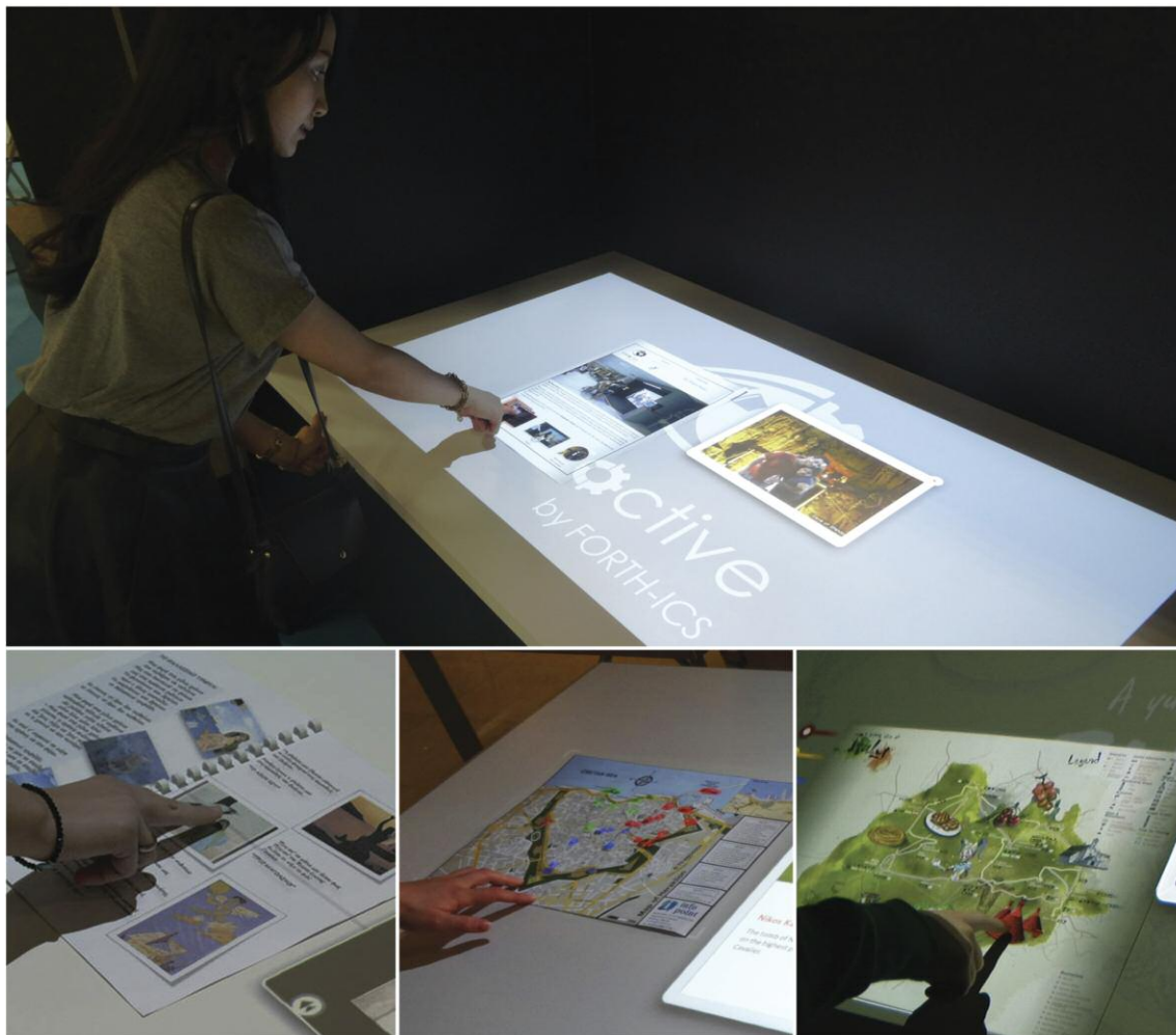
Figure 1: User interaction with augmented printed documents. Main: the system highlights regions of potential user interest; upon user touch, relevant content is augmented, juxtaposed to the document. Thumbnails: multimedia augmentation in a music and poetry book (left), map augmentation providing city tour information on the printed map (middle) and visitor information (right).
