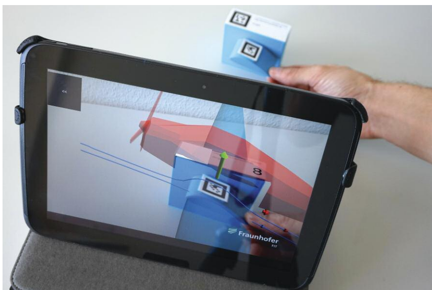
Figure 1: Visualizing forces and airstreams around a miniaturized wing using Augmented Reality.
