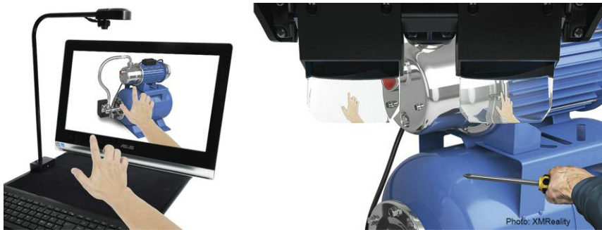
Figure 1: The AR equipment. A screen together with a camera pointing downwards for the guide (left) and a pair of HUD goggles with a front facing camera for the follower (right).
