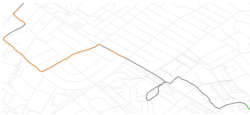
Figure 2: Road environment types – namely, downtown (orange line), industrial/commercial (dark grey line), and residential (green line) environments – inferred by a modular full ANN along a route in Csepel, Hungary. (Map data: OpenStreetView, map-editor: QGIS 2.8.1.)
