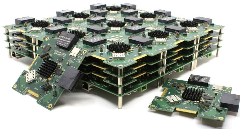
Figure 2: The SCALP platform, a set of FPGAs and processors with 3D topology, was designed to evaluate self-organisation mechanisms on cellular machines. Algorithms based on cellular self-organising maps are the basis of the self-adaptation properties.
