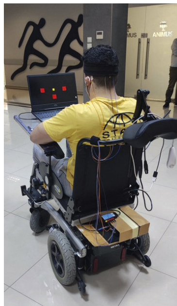
Figure 1: Evaluation of the SSVEP-based BCI for wheelchair navigation at ANIMUS Rehabilitation Center.
