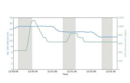
Figure 1: (A) Test setup with UAV hovering above gas basin. (B) Measured  $CO_2$  concentration at varying hover altitude in response to CO2 bursts from a fire extinguisher. Blue line (lhs): UAV altitude; Green line (rhs): CO<sub>2</sub> concentration; Shaded areas: Duration of  $CO_2$  bursts.
