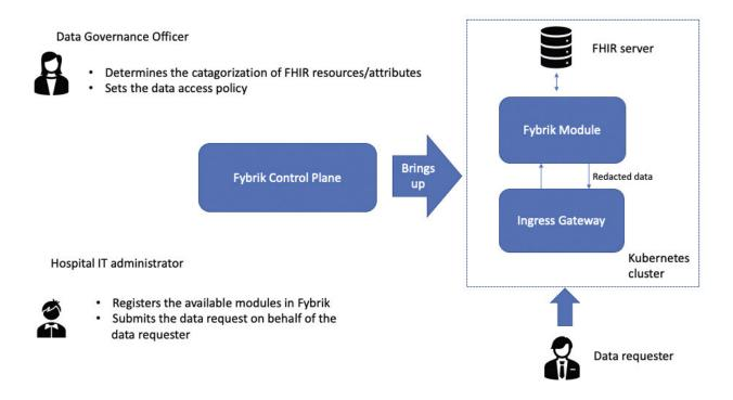
Figure 1: Use of Fybrik to create a PAF.
