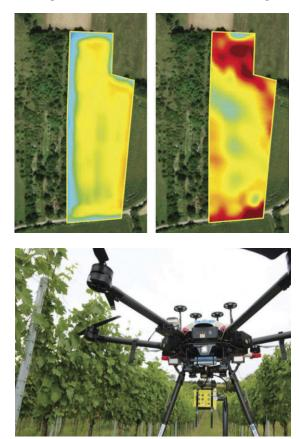
Figure 1: Precision farming system – (top) sensed microclimate conditions visualiszed by different colours in a vineyard and (bottom) scanning drone [1].
