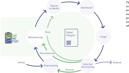
Figure 1: Battery life cycle, accompanied by a digital product passport. BatWoMan uses manufacturing data generated in the project and external/estimated data for other life cycle phases.
