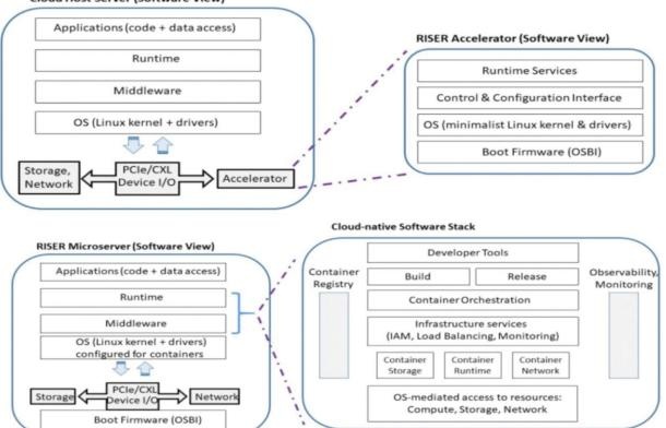
Figure 2: System software for the two RISER platforms: accelerator interacting with host, and microserver with cloud software stack
