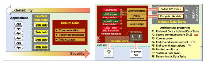
Figure 1: ES-PDMS logical architecture and a concrete implementation [L2].
