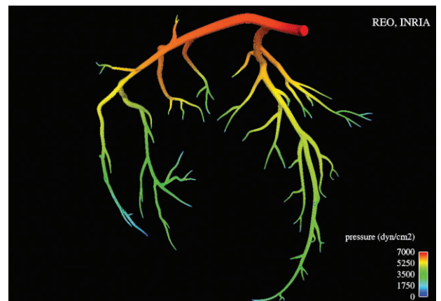
Pressure field of a steady flow in a left coronary network (rigid wall; motionless vessel axis) using fluid solver LifeV. Pressure inlet condition; traction-free outlet condition to be coupled to a perfusion model in a porous medium (from JF. Gerbeau, G. Rossi and I. Vignon-Clementel).
