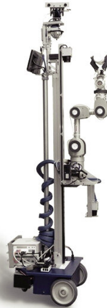
Figure 5: The robot E-LE developed at Georgia Tech for studies of assistance to elderly/disabled people (Courtesy of Prof. C. Kemp, RIM@GT).
