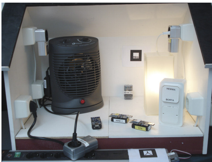
The smart house demo consists of several sensor nodes measuring temperature, light and power consumption. This data is used as input to the control system. All sensor data is collected over an IPv6 network.
