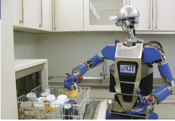
ARMAR-III, a humanoid robot of the Karlsruhe Institute of Technology developed by the Collaborative Research Center on humanoid robots (SFB 588), funded by the German Research Foundation (DFG), as assistance robot in human-centered environments.
