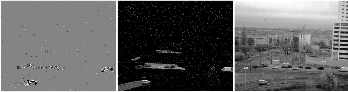
Figure 2. Temporal contrast change events, change-triggered exposure data starting from an empty image, and continuous-time video stream. The event-based video contains the same information as standard frame-based video at data rates reduced by orders of magnitude.
