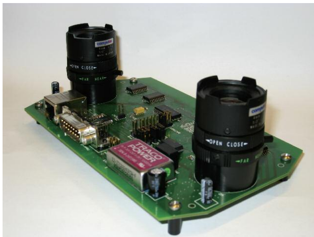
Figure 1: Image of the event-based stereo vision system.
