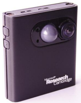
Figure 2: The SenseCam provides passive image capture, enabling increased contextual cues.
