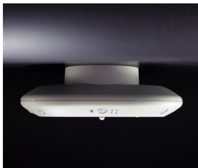
Figure 2: A multisensory node with several motion sensors.
