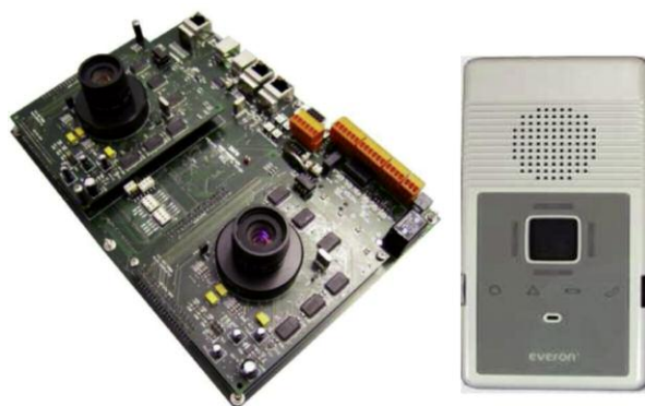
Figure 1: CARE key technologies: Stereo vision system for fall detection (left), Everon wireless module (right).
