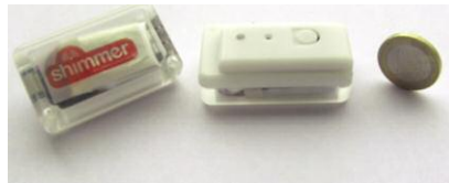
Figure 1: The SHIMMER unit can be worn around the ankle and measure gait.
