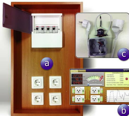
Figure 2: (a) Simulation box with electrical panel and four plugs, (b) application for control and monitoring and (c) circuit for retrieving data wirelessly.
