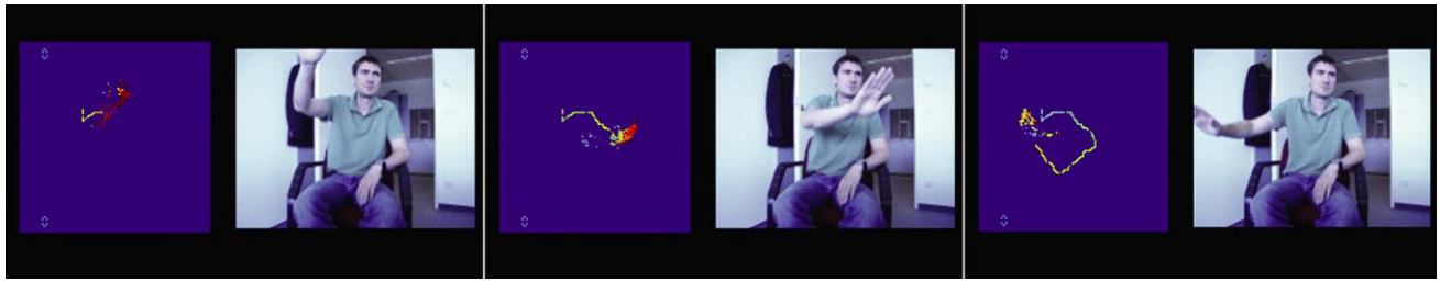
Figure 2: A sequence of still images provide an example of raw hand tracking data (left pane) and synchronous video (right pane) for a person performing a “circle” gesture.
