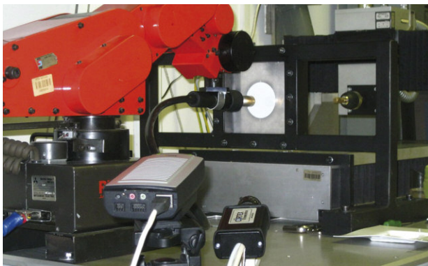
Figure 4: FANUC S-430iF robot, lights-camera box and Rubik's Cube
