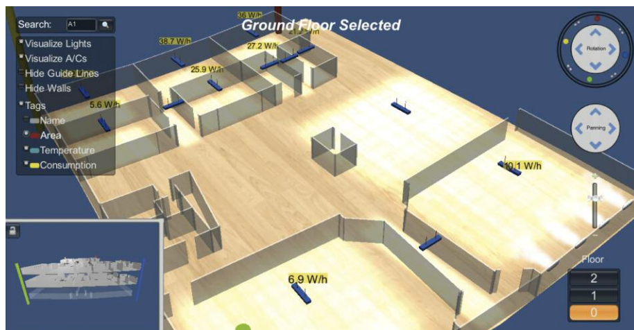
Figure 1: Screenshot of the VRE prototype application displaying energy data and rendering status of devices at INESC-ID Taguspark building
