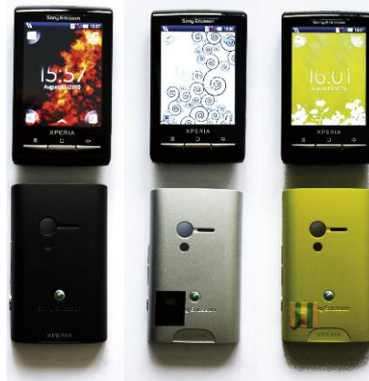
Figure 1: Mobile phone prototype using magnets on shells to control themes and other content.
