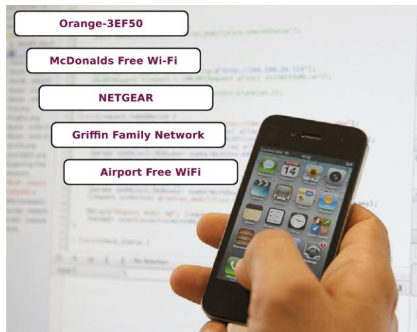
Figure 1: A smartphone broadcasting in plaintext its Wi-Fi fingerprint, ie names of networks to which it has previously been connected.
